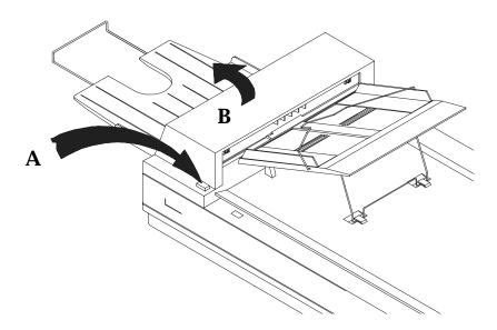
Figure 4.1 ADF Paper Jam - Opening the ADF.
